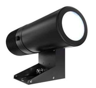
A very powerful LED projector designed specifically to project signs in harsh industrial environments. The absence of fans and a degree of protection of IP65 means it can be used in dusty places, both indoors or outdoors, for extended periods of time, with an average LED life of 50,000 hours.
